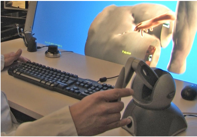
Figure 3: Virtual palpation by sliding a virtual hand over the skin surface with visual display of underlying landmarks.
